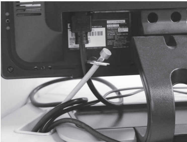
FIGURE 10.10 If theft of equipment is a possibility, run one end of the cable from the monitor to the desktop machine through the hole in the work desk.
