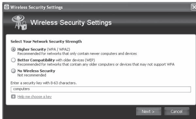
FIGURE 5.2 Wireless security settings for a simple router
