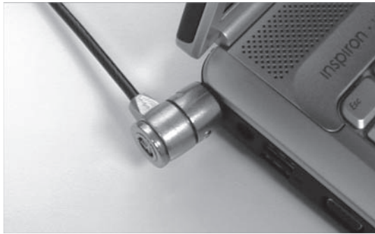
FIGURE 10.8 A cable in the security slot keeps the laptop from easily being removed.
